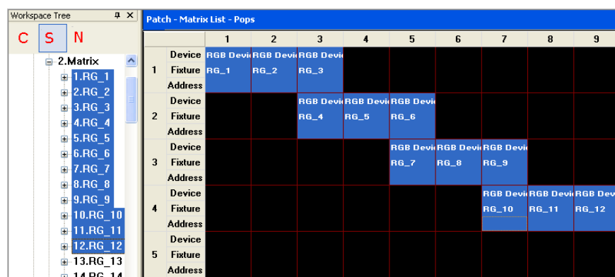
Figure 115: Mapping fixtures to selected cells
