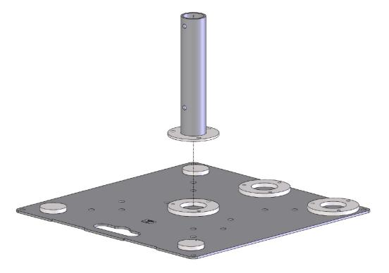
II. Fit the three M10 x 20 long screws (grade 8.8) along with the washers provided. (All three screws must be fitted). See section 13 for fixing part numbers.
