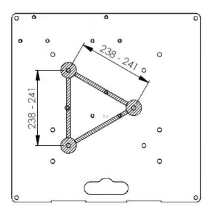
Tank Trap used as a truss base showing the positions of 238mm - 241mm triangular truss sections.
