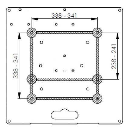
Tank Trap used as a truss base showing the positions of 338mm - 341mm square sections.
