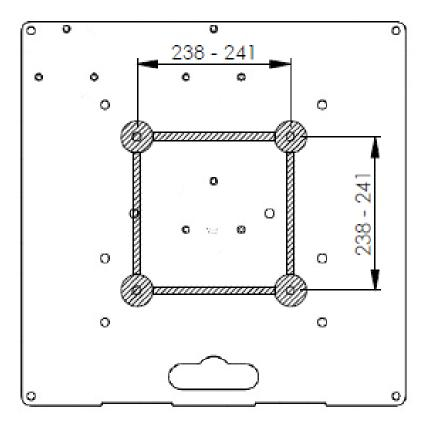
Tank Trap used as a truss base showing the positions of 238mm - 241mm square truss sections.
