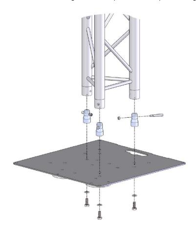
Tank trap base plate used as a truss base-plate.
