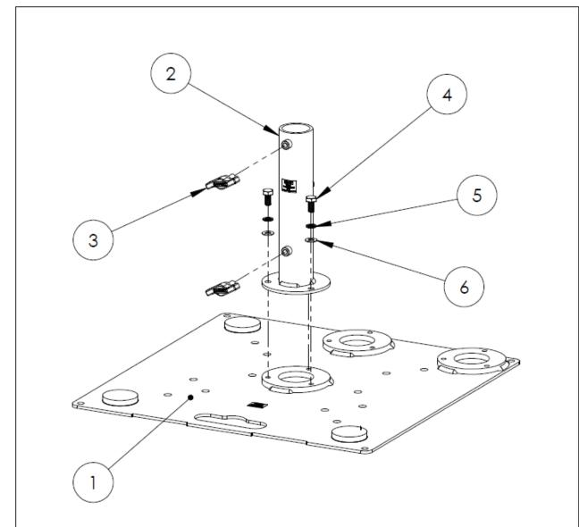
FIXINGS F892, F902 & F994 CAN BE ORDERED AS A SET (3 OFF EACH PART) UNDER PART NUMBER S3641
