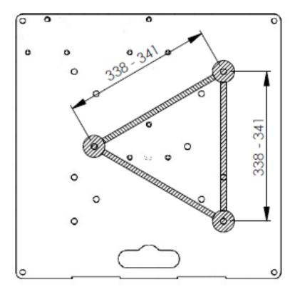
Tank Trap used as a truss base showing the positions of 338mm - 341mm triangular truss sections.
